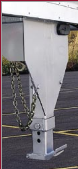
Standard AWG/AWGA Hitch (2 5/16" Adjustable Height Ball Hitch)
